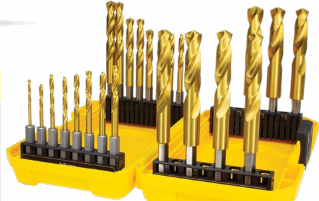
135° Split Point Cuts faster and reduces wandering
